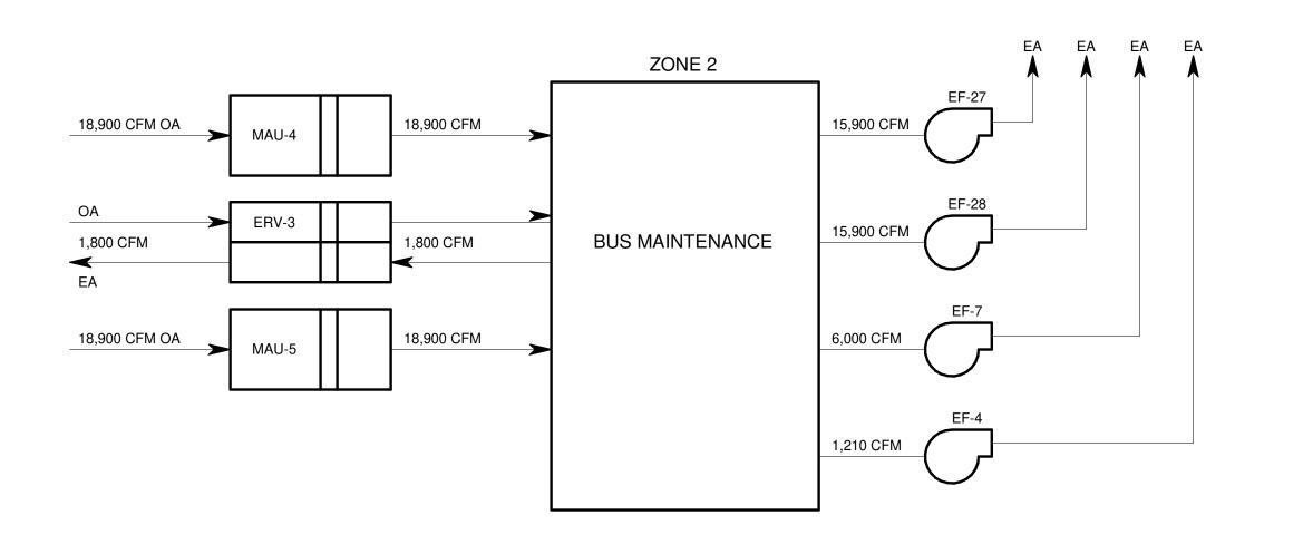
BUS MAINTENANCE AIRFLOW DIAGRAM
