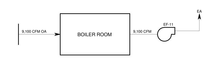
7 BOILER ROOM VENTILATION AIRFLOW DIAGRAM
